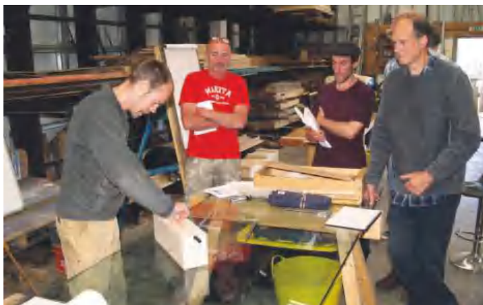
▲ Pic.1 Japanese carpentry works on centrelines. The first job, once all the timber has been squared up, was for Mathieu to snap a centreline using a sumi-sashi ink line. We used American tulipwood from Sydenhams timber yard, Maiden Bradley, because it is stable and clean. More about marking out can be found on Mathieu's blog: https://fabulalignarius.wordpress.com/2015/05/
